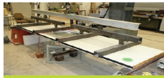
Fig.3 Testing strength of panel with window frame installed
