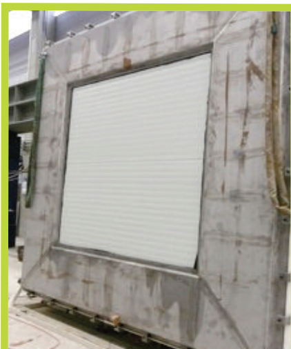
Fig. 1 Test setup for measuring air leakages through panel joint. Technische Universität Darmstadt
